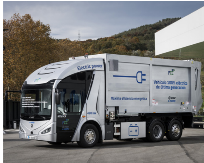
Side-loading electric collection vehicle developed on the FCC e-mobility platform.
