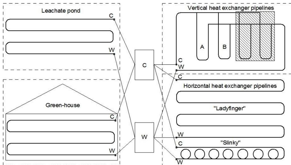
Figure 1. Schematic of the built technological system. (C - cold, forward pipe; W - warm, backward pipe).
