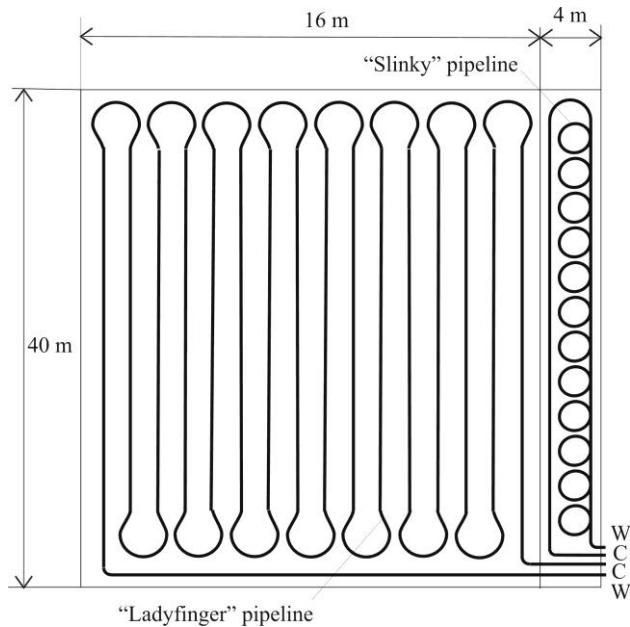
Figure 2. Plan of the horizontal heat exchanger pipelines (W – warm, C – cold).
