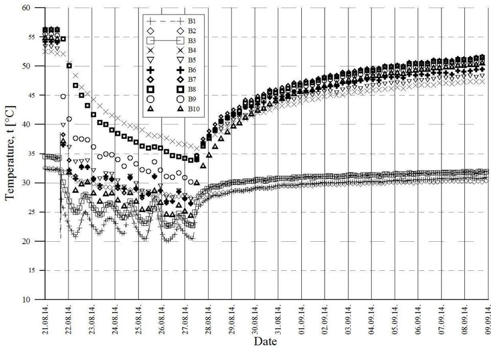
Figure 8. Measured temperatures in heat well B as function of time.
