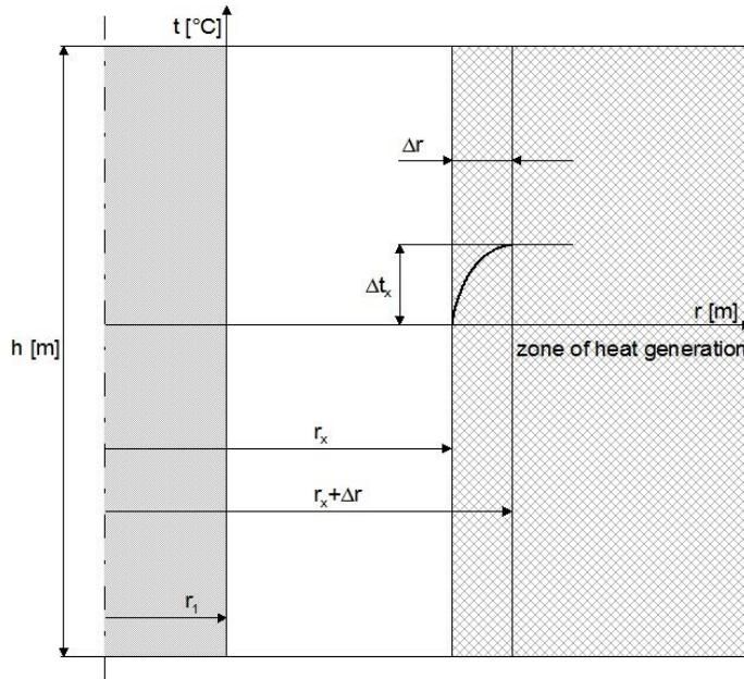
Figure 11. The „tube shell with heat generation” model.
