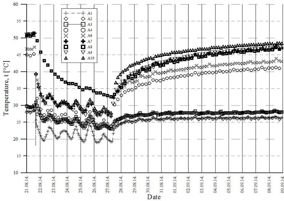
Figure 7. Measured temperatures in heat well A as function of time.
